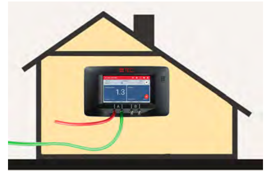
Figure 1. Measuring pressure of house main body with reference to (WRT) outside.
