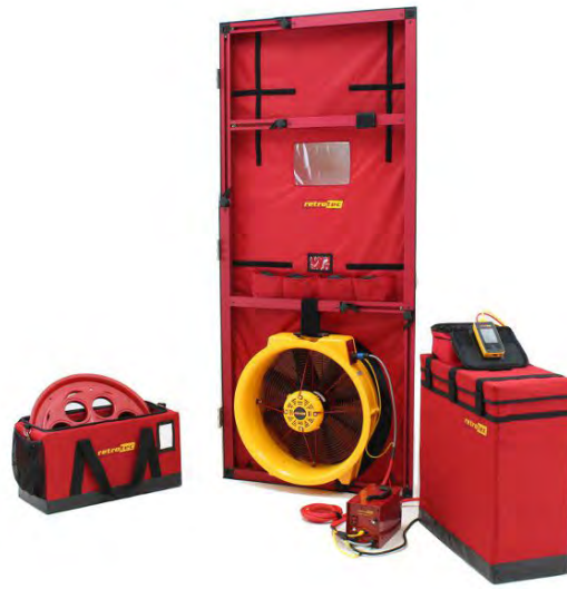
Blower door set up for an air leakage test. Photo: Retrotec
